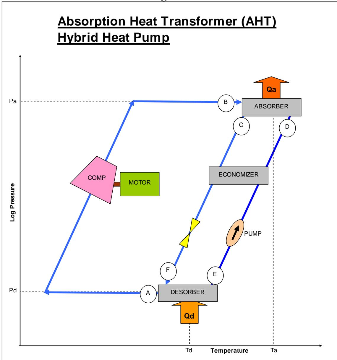
entering the desorber at line (F). The resulting weak liquid solution leave the desorber at line (E), to be pumped to higher pressure, ( $P_a$ ) of the hot absorber. The pumped NH<sub>3</sub>-lean solution line E -> D is also in heat exchange (economizer) contact with the NH<sub>3</sub>-rich solution line C -> F flowing from the hot absorber back to the low pressure ( $P_d$ ) cold desorber.
