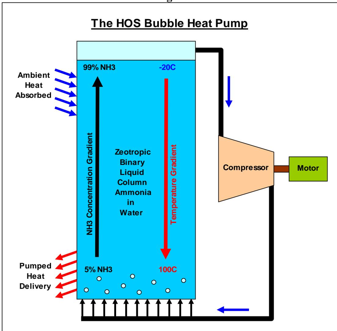
from 5.85 Bar Abs to  $P_a = 1.99$  Bar Abs, (with the reduction of  $NH_3$  concentration in the absorber to 15.19%  $NH_3$  in aqua from the previous 32.89%), resulting in the real
