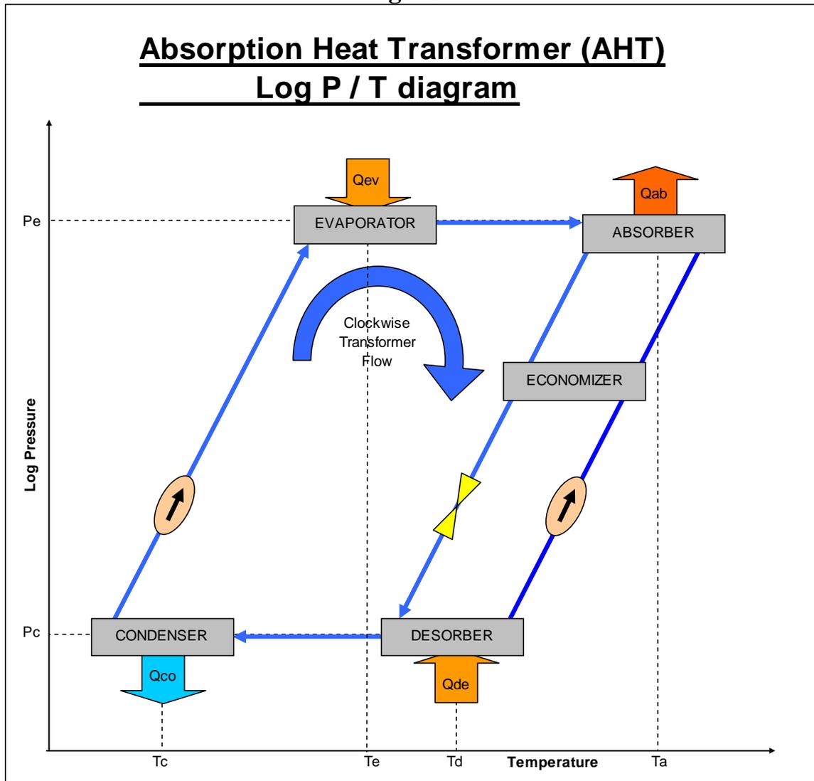
heat input into the desorber as ( $Q_{de}$ ) at temperature  $T_d$ , and intermediate temperature heat for the evaporation process as ( $Q_{ev}$ ) at temperature  $T_e$ . The high temperature output heat is shown as ( $Q_{ab}$ ) from the hot absorber at temperature  $T_a$ .
