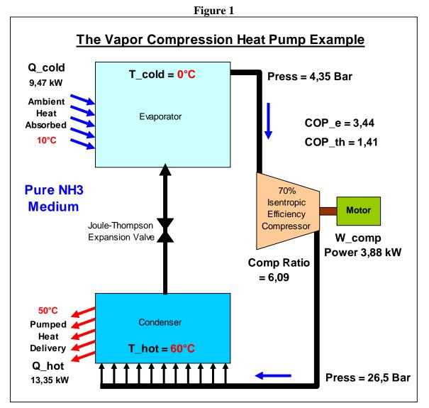
The electrical coefficient of performance (COP\_e) for cooling service is defined as:
