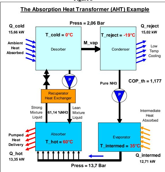
example sketched in figure 3, ammonia vapor saturated at 35°C is generated in the evaporator and is absorbed in the absorber (and heat it with the absorption heat) to 60°C, matching the 13,7 Bar pressure of the evaporator. The saturation vapor pressure of pure NH3 at 60°C is 26,5 Bar, double the actual absorber pressure, demonstrating the huge pressure reduction achieved by using an absorber instead of condenser.
